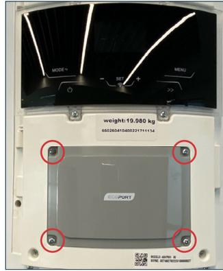
**4.** The EcoPort cover is now exposed. Remove the 4 screws using a Phillips head screwdriver in the corners of the plate to remove the plate.
