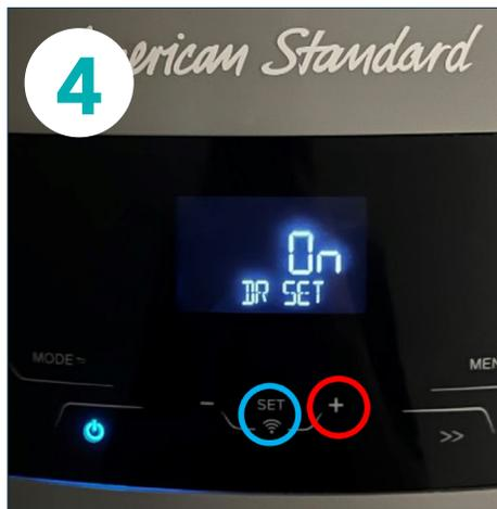
3. Using the "+" button, navigate to P37 "DR SET" and click the "SET" button on the control screen.
