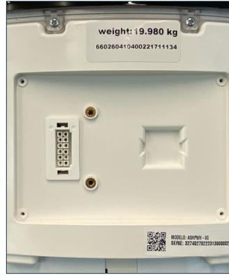
**5.** Remove the plate to expose the EcoPort. The EcoPort will be exposed and have several prongs in two columns on the left, two screw holes in the middle, and a square shaped indent on the right.
