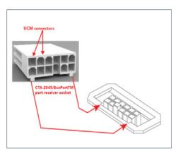
Plug the UCM into the CTA-2045/ EcoPort<sup>™</sup> port receiver socket by aligning the UCM connectors with the connectors of the CTA-2045/EcoPort<sup>™</sup>. Gently push in the UCM until the bottom face of the UCM touches the flat face of the receiver.
