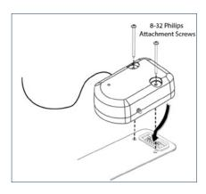
In most cases, the screw sockets on the UCM will align with the screw sockets on the CTA-2045/EcoPort™. If this is the case, use the screws to secure the UCM to the receiver.
