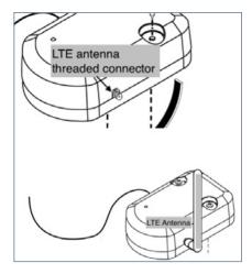
4. Point the LTE antenna up and away from the water heater. Based on your water heater configuration you may need to bend the antenna up or rotate it away from the water heater. Be careful when doing so.
